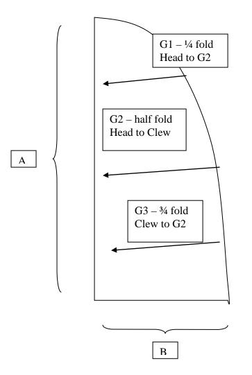
A and B entered into Measurement Certificate. Size + Max Headsail size placed on Port side. Max Headsail = 18.58 – Mainsail M2.
